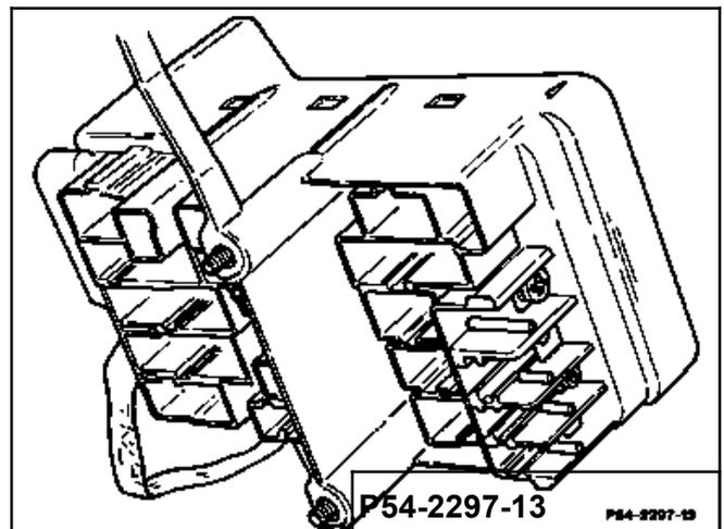
The terminal 30 (arrow) is fed in at the front face of the central electrics. As of 10/85 the terminal 30 is held by an M6×10 combination screw. Further connections are possible on terminal 30, terminal 15 and terminal 15 R.
