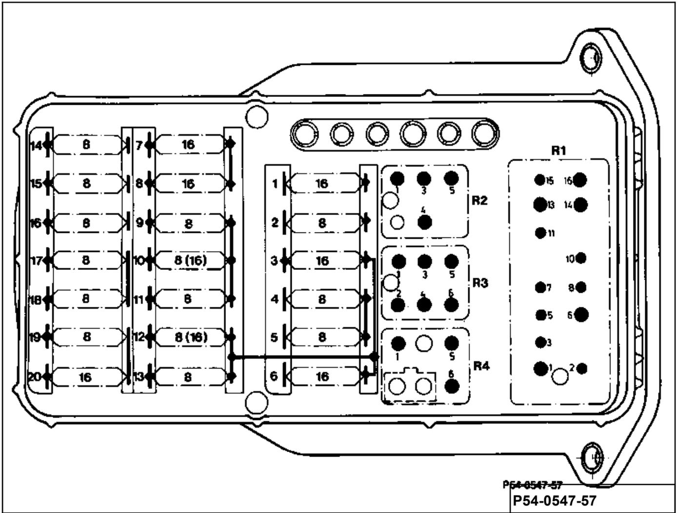
Assignment of fuses see insert sheet in cover of central electrics.
