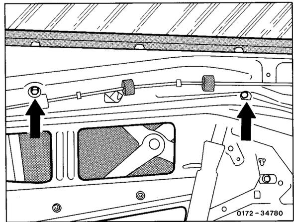
10 Close crank window and adjust rear guide wedge by sliding in oblong hole so that the rear edge of the window contacts the guide wedge.
