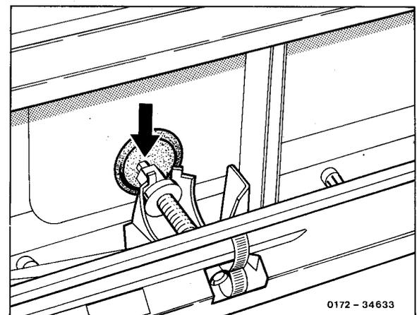
12 Remove rubber grommets and loosen nuts. Adjust crank window with both adjusting screws in such a manner that, with the window closed, the upper edge of window pane is just resting against sealing frame when the door engages in 1st detent of door lock.
