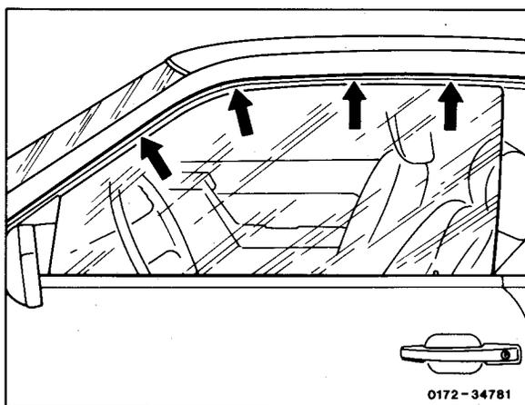
8 Tighten nuts on upper angle stops front and rear.
