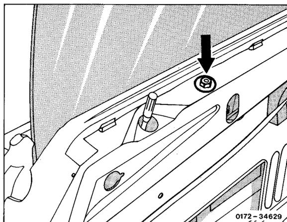
14 Adjust lower lift restriction with stop against window lift and on window lifting rail in such a manner that the upper edge of the window pane is flush with sealing rails.
