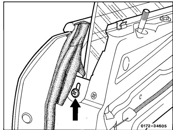
11 Adjust lateral tilt (preload) of crank window in relation to sealing frame by means of adjusting screws on front and rear bearing bracket of vertical guide rail. For this purpose, remove trim outside on driver's door (88-800, section B).
