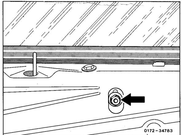
6 Close crank window until crank window is flush with front edge to guide holder.
