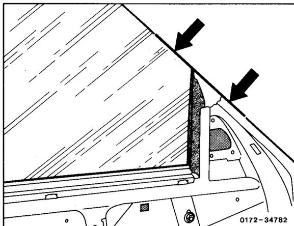
7 With window correctly adjusted, the upper edge of glass will touch the inner lip of sealing frame along entire length.
