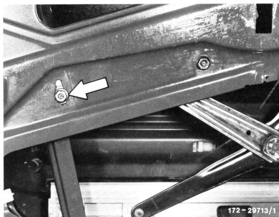
9 Tighten front nut on guide rail.
