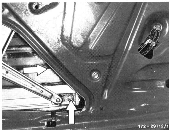
8 Push rear nut on guide rail down and tighten.
