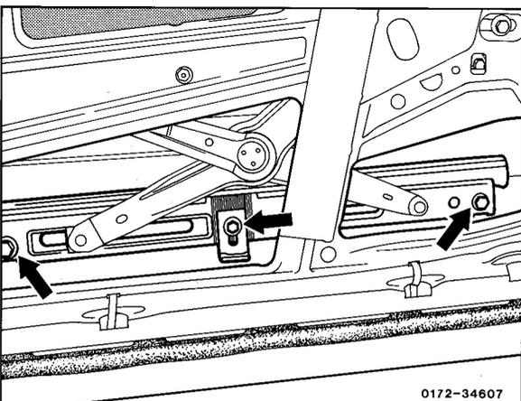
9 Tighten front and rear screw on window lifting rail.
