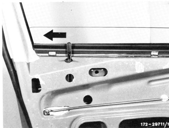
7 Push window below in forward direction into window running rail and tighten nut on window lifting arm.
