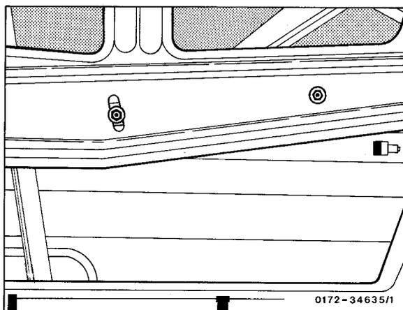
If required, the tilt and the longitudinal direction of crank window can be additionally corrected after loosening the three screws on window lifting rail.
