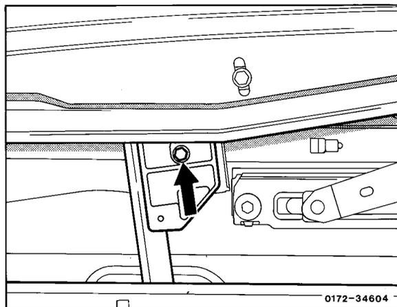
13 Adjust rear guide rail in slot in such a manner that the rear edge of the crank window abuts against sealing rubber of rear side window along entire length with door closed.
