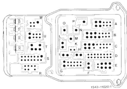
13 Connect the black line from the auxiliary harness (central electric system) on one of the terminals 15 and the red line on one of the terminals 30 of the line connector.
