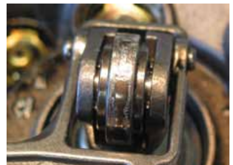
Damage: Cam roller with pittings due to worn cam disk.
