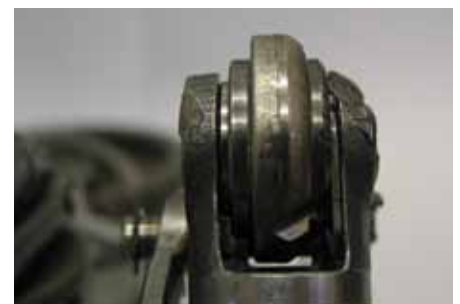
Damage: one-sided wear on the cam roller
