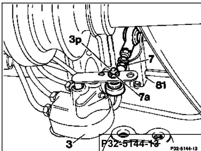
3 Connect oil drain hose (061) to oil drain plug (3p) on level controller.
