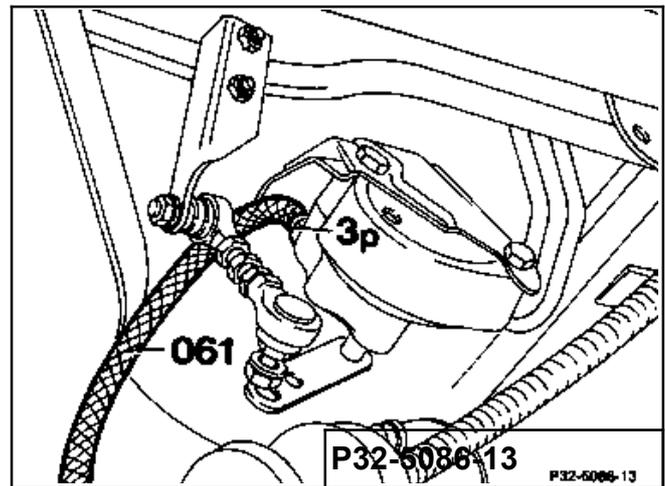
6 Connect pressure tester (038) with test hose (038g) to level controller (3).
